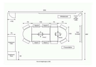
**Fig. 1.** The layout of the UEDIN Instrumented Meeting Room (measurements in cm). Array microphones are numbered 1-16. Cameras are mounted under Array 1 to give closeup views of participants in the seated locations. The six reading locations are indicated as Seat 1-4, Presentation and Whiteboard.
